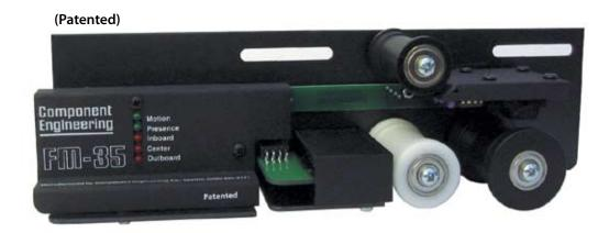
The FM-35 Cue Detector provides all of the outputs required by today's theatre automation. It includes three separate proximity sensors for foil tape cue detection and four optical sensors for the monitoring of film presence and motion across the film frame. The outputs are conditioned to provide proper cue pulse lengths and eliminate false dropouts on splices.
