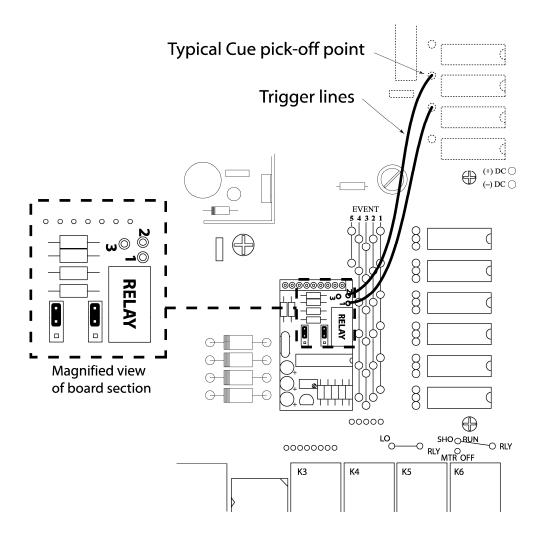
The adjustment of the timer is mostly a "set and try it" proposition. With the machinery running, initiate a lens change which will also close the douser and start the timer. Note when the douser opens again and adjust the timer to suit. Turning the timer control counter-clockwise will shorten the time. You are finished!
