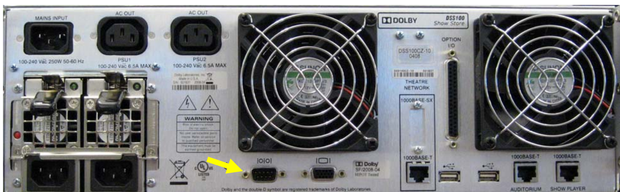
Figure 9: Serial Communications Port on a Dolby Digital Cinema Server
