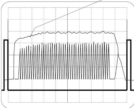
Many small saw teeth indicate correct LED vertical adjustment.
