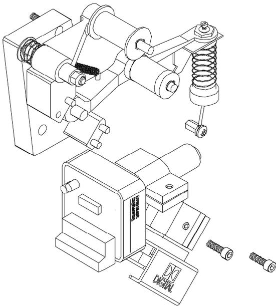
The **dual lens/pre-amp assembly** should now be carefully eased onto the dowel pins in the adapter block and bolted in place. It is a good idea to have the digital video cable already plugged onto the digital pre-amp circuit board before you mount this assembly.
