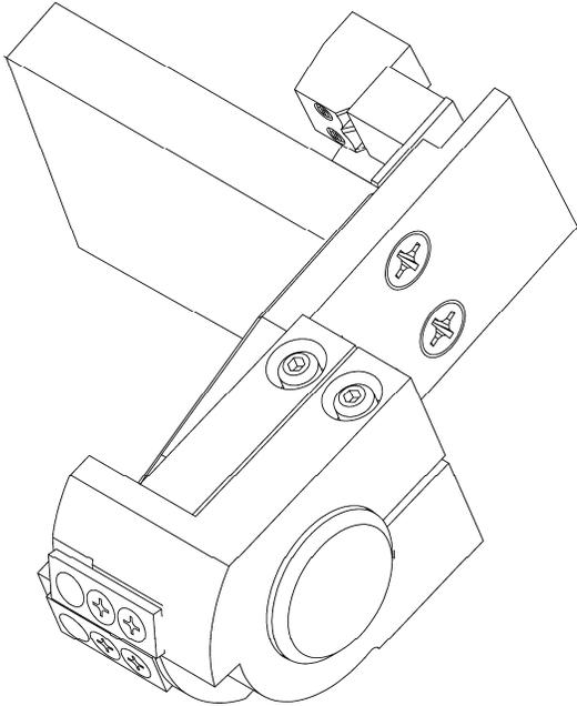
The **LED assembly** can now be mounted to the top of the standoff post by means of two 4-40 Flat Head screws.
