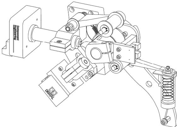
Attach the plunger of the AirPot to the standoff on the locator plate. Leave the nylok screw loose enough so it will not bind the plunger.
