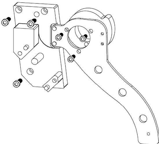
Position the locator plate's large hole over the sound drum's ball bearing seat and hold in place with three 8-32 x 1/2" screws through the holes on the right side of the plate. Do not tighten these screws.
