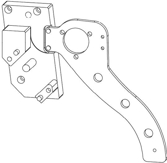
As you begin the installation please refer to the drawings on the left. Assemble the locator plate and adaptor block by slipping the 2 holes in the locator plate over the 2 pins in the adaptor block.
