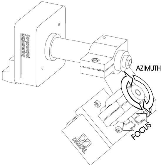
Rotation of trace indicates incorrect reader azimuth adjustment.
