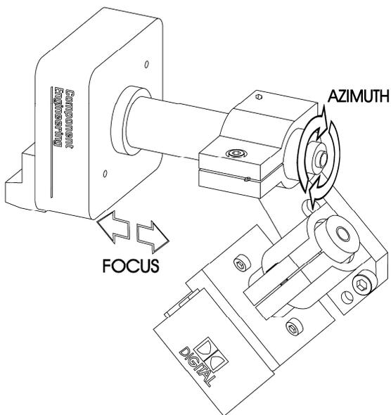
**Analog focus and azimuth alignment**
