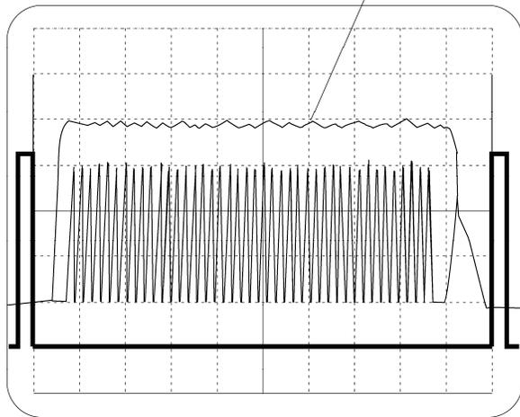
Azimuth adjustment is difficult when using only a 'scope. Rotate the reader to adjust for the flattest perf trace and the lowest error rate on the processor display. Large azimuth errors are seen as a tipping of the 'scope sprocket hole trace. The axis will be the center of the displayed perf trace. The DRAS azimuth number you are looking for is as close to zero as possible. Retighten the clamp screw when both focus and azimuth have been optimized.
